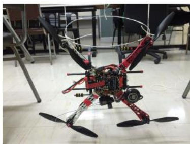
Figure 3. Measurement of Moment of Inertia along the y-axis.
