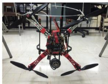
Figure 2. Measurement of Moment of Inertia along the x-axis.
