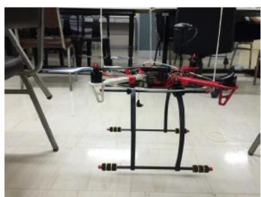
Figure 4. Measurement of Moment of Inertia along the z-axis.
