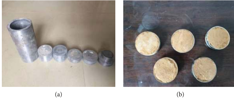
FIGURE 6: Preparation of remolded loess sample.
