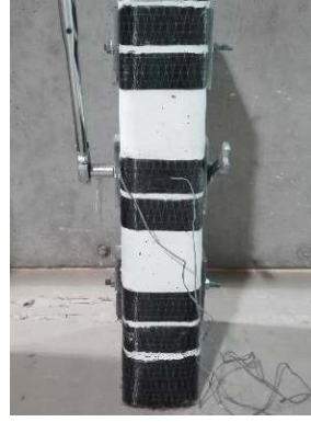
Fig. 3 - Representation of the prestress application on the CFRP strips
