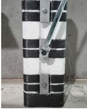
Fig. 3 - Representation of the prestress application on the CFRP strips
