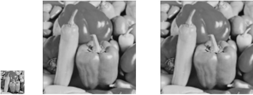
Fig. 4. The LR 128 \times 128 input image, left, the 512 \times 512 image reconstructed by bilinear interpolation, middle, and by the improved algorithm, right
