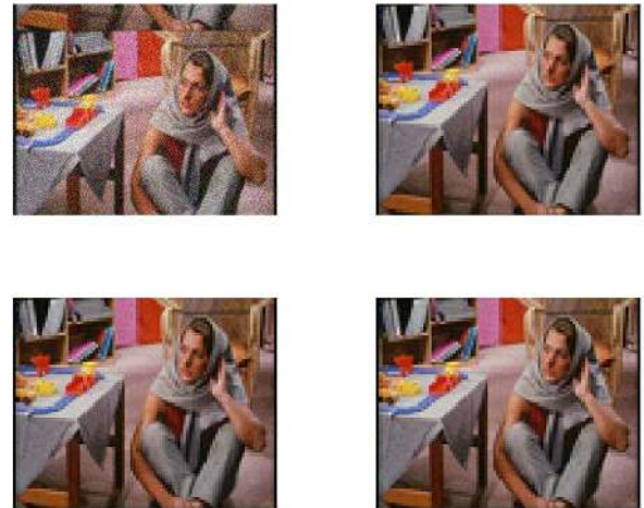
FIGURE 7. The blurred image (top left), the restored image by Algorithm 1 (top right) (SNR= 13.67, PSNR= 20.09, SSIM = 0.6289), by Algorithm 2 (SNR = 13.65, PSNR = 20.07, SSIM = 0.6277) (bottom left) with and by Algorithm 3 (SNR = 13.66, PSNR = 20.08, SSIM = 0.6285) (bottom right).
