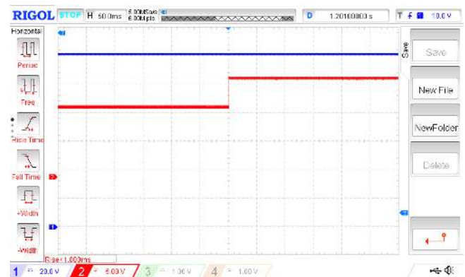
FIGURE 32: Effect of Change in V_{in} from 12V to 17V on V_o
