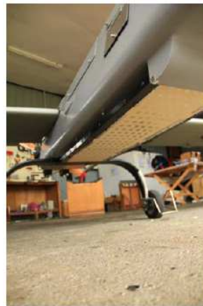
Figure 15. The SAR antenna mounted at the bottom of the UAV's fuselage.
