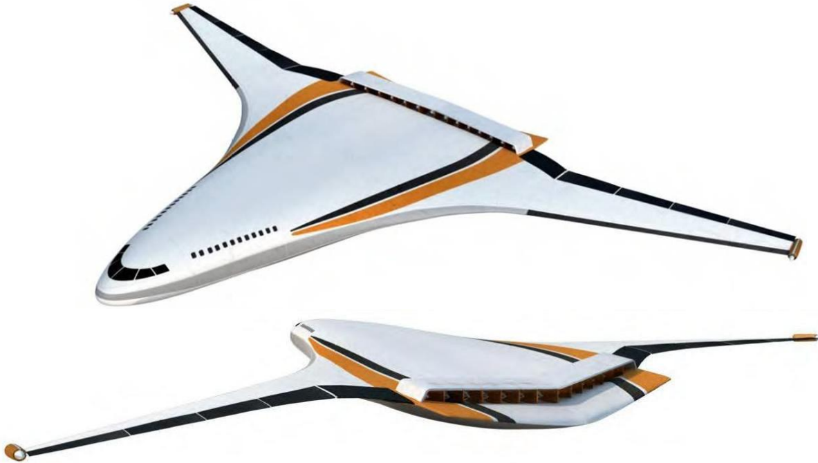
Figure 1. Two views of the N3-X vehicle as envisioned in References 1-6, showing the arrangement of propulsors and wingtip-mounted turboshaft engines (Graphics: NASA).
