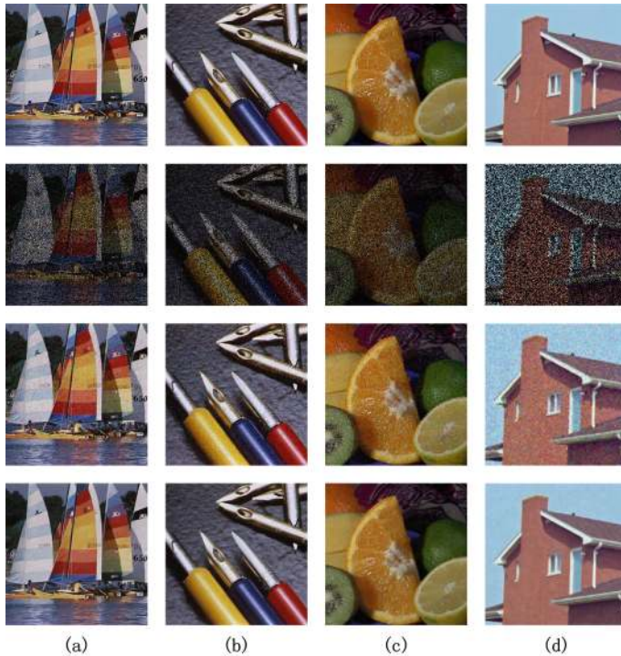
Fig. 6. From top to bottom: original images, corrupted images, pre-completion results and the recovered results of our approach. The damaged images here have a higher missing rate of 60% and \sigma = 25 . The PSNR values of the recovered results in (a), (b), (c) and (d) are 28.37dB, 30.35dB, 28.64dB and 30.62dB respectively.
