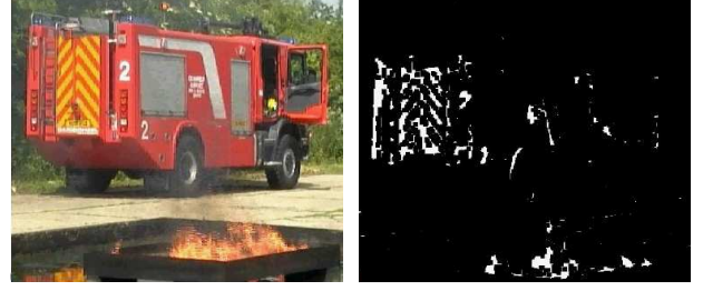
Fig. 3. Original image (left) and corresponding fire pixels regions detected using colour spectroscopy (right).
