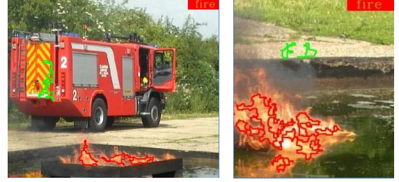
Fig. 4. Fire pixels regions detected using 2-stage colour spectroscopy and decision tree classification (red), single-stage colour spectroscopy only (green)
