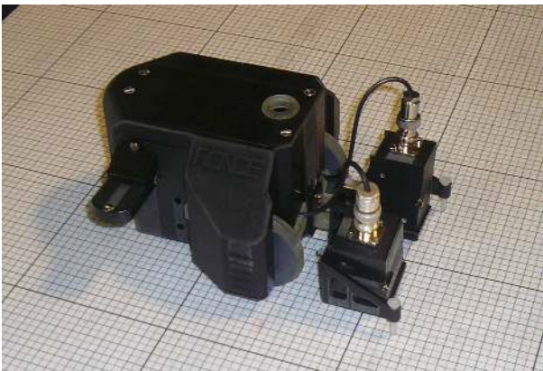
Fig. 2. Ultrasonic inspection robot showing air-coupled ultrasonic payload. The bold lines have 100mm spacing.
