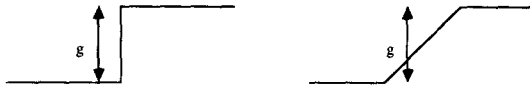
FIG. 8. Edge profiles: (a) an ideal step edge; (b) an ideal ramp edge.
