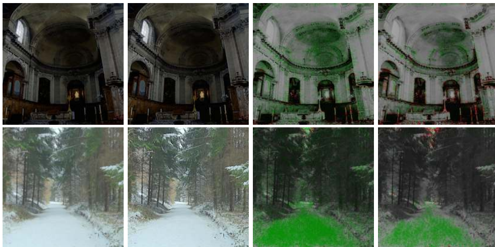
FIG. 4.2. Evaluation of preprocessing stage for Ferradans et al.[11] (top row) and Drago et al. (bottom row) TMOs. From left to right: input tone mapped image, output of preprocessing stage, distortion map of the input, distortion map of the output.
