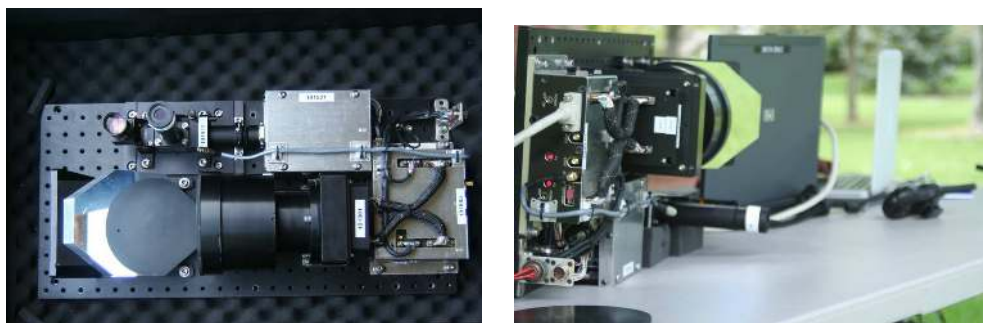
Figure 3.1. (a) ASC Portable Ladar Camera mounted to machined brass plate, in storage box. (b) Camera deployed for collecting images
