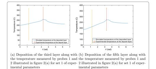
**Fig. 6** Comparison of the simulated temperature in the middle of the top layer, with experimental measurements, for the 3rd and 5th layer deposition. Temperatures in °C
