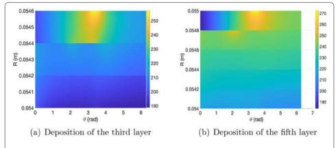
$\textbf{Fig. 5} \quad \text{Vertical section in the deposited layers during the deposition of the 3rd and 5th layers.} \\ \text{Temperatures in } ^{\circ}\text{C}$
