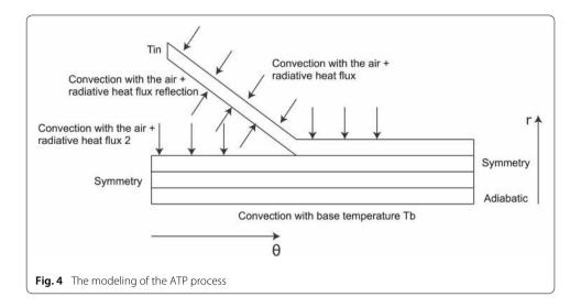
of the temperature between ply l at  $\theta = 2\pi$  and ply l-1 at  $\theta = 0$ . The tip of the very first layer is considered adiabatic. The boundary conditions are reviewed in Eq. 14.
