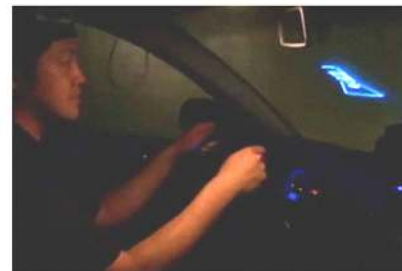
Fig. 2. LISA-P test bed. DAD display capabilities and limitations and the approximate location of alerts used for the speed control experiment. Within these limitations, the DAD is capable of drawing anywhere on the windshield.
