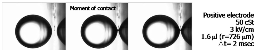
FIG. 1. Moment of contact: The drop can be charged by direct contact, by transfer of charge along an electrically conducting path, or by both mechanisms.
