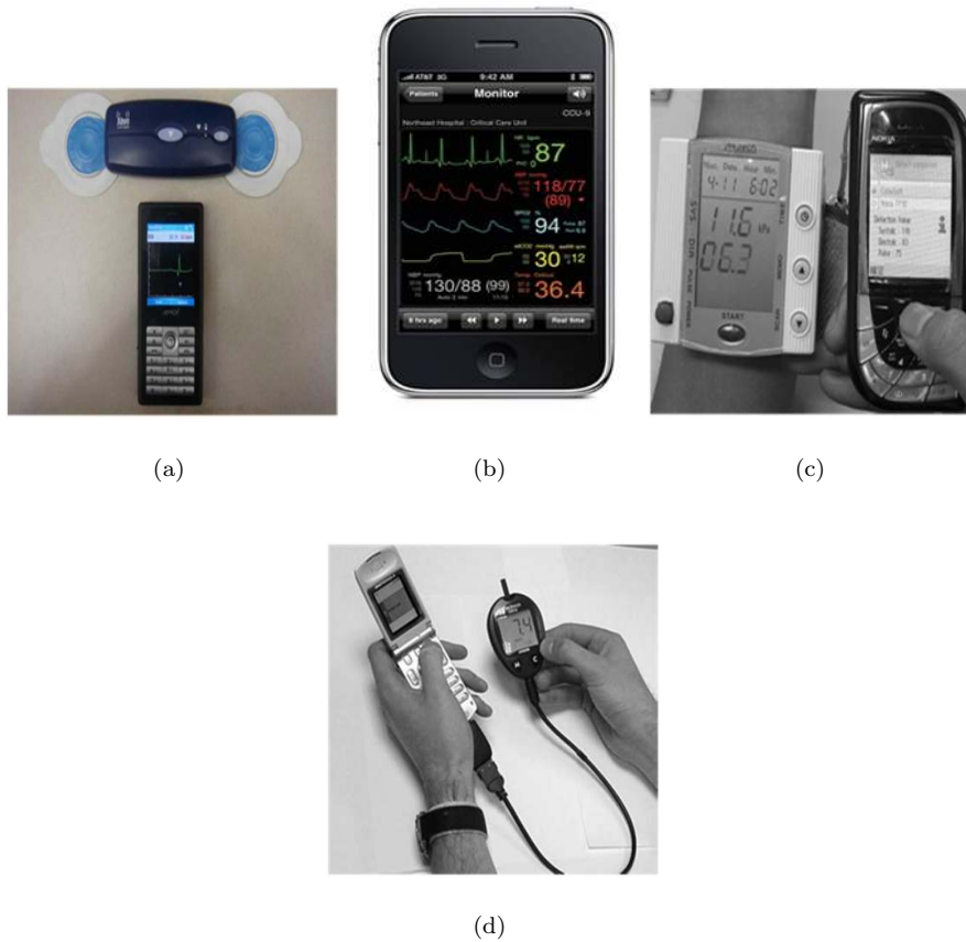
Fig. 2 Health care applications uses Smartphones to monitor (a) ECG, (b) Blood pressure, heart rate, SPO2, and body temperature (c) Blood pressure and Pulse (d) Blood sugar level.
