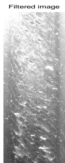
Figure 2. Filtered heavy RCF damaged rail (NRC, Canada)
