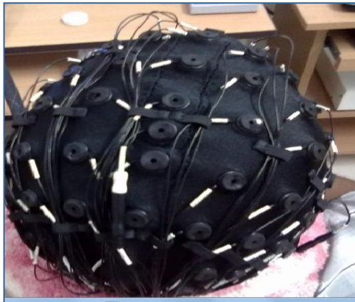
Fig.6. Participant wearing the EEG cap with 64 electrodes plugged
