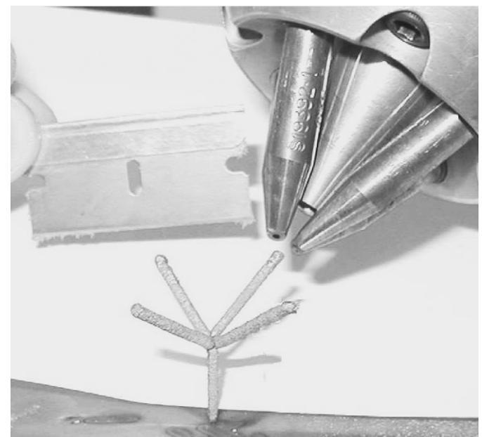
Fig. 10. A branched structure with linear segments fabricated by laser-based direct metal deposition.
