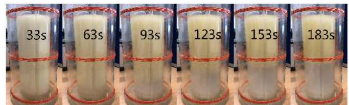
Fig. 15. Screenshots from the recorded video during the separation process.
