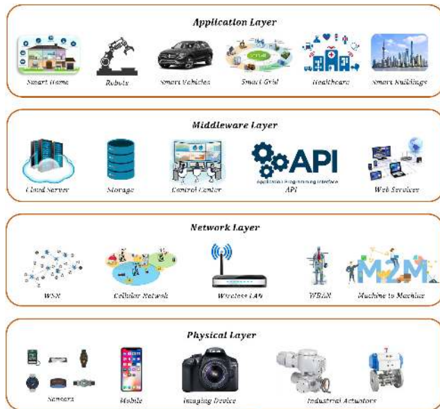
FIGURE 1. Industrial IoT system architecture.
