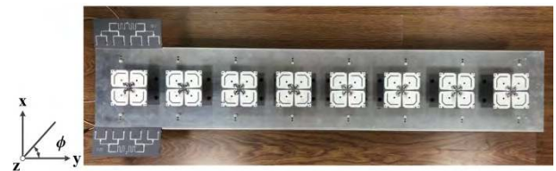
FIGURE 15. Prototype of linear array with the BEDPA.
