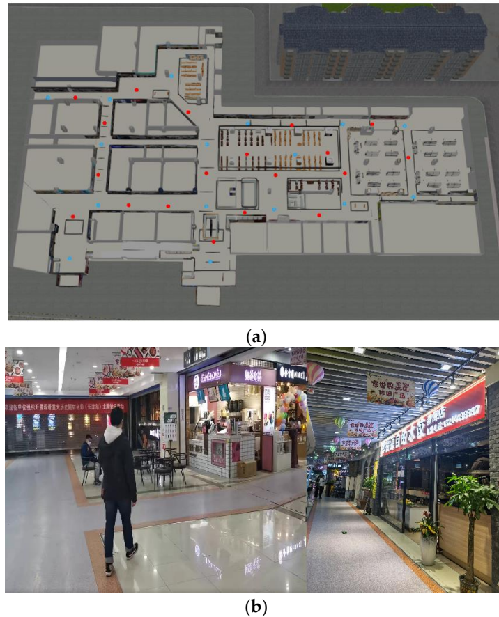
Figure 12. Test scenario. (a) is floor plan of the mall. The blue point is the location of the communication-positioning integrated base station, and the red point represents the test point. (b) is a photograph of the test scenario.
