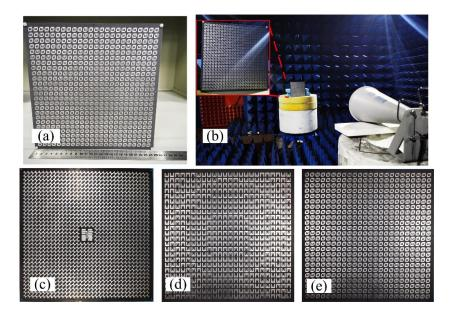
**Figure 12.** (a) The fabricated GCPFTA. (b) The measurement of GCPFTA in anechoic chamber. (c) The integrated reflectarray and planar feed antenna with total size of 238 mm  $\times$  238 mm  $\times$  2.5 mm. (d) The E-shaped patches on the bottom layer of transmitarray with size of 240 mm  $\times$  240 mm. (e) The anisotropic patches on the top layer of transmitarray with size of 240 mm  $\times$  240 mm.
