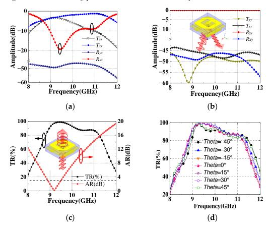
**Figure 3.** The reflection and transmission amplitudes of the unit cell under (**a**) *x*-polarized and (**b**) *y*-polarized incident waves. Simulated (**c**) AR and (**d**) TR under *x*-polarized incident waves.
