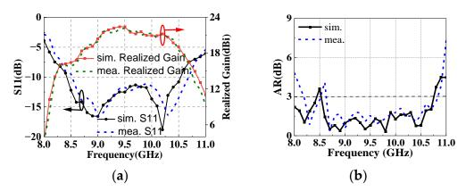
Figure 16. Simulated and measured results of NCPFTA (a) S11, realized gain and (b) AR.
