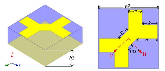
Figure 6. The schematic geometry of reflectarray unit cell.
