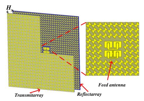
Figure 10. The schematic of GCPFTA.
