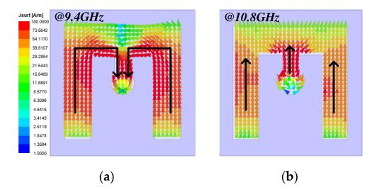
Figure 4. The current distributions on bottom E-shaped patch at (a) 9.4 GHz and (b) 10.8 GHz.
