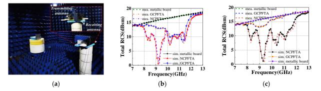
band. For *y*-polarized detection waves, the NCPFTA shows obvious RCS reduction at 7.7–12.7 GHz. Compared with GCPFTA, the maximum RCS reduction is 12.9 dB at 9.4GHz.
