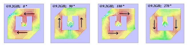
**Figure 5.** The current distributions on top anisotropic patch with phases of  $0^\circ$ ,  $90^\circ$ ,  $180^\circ$  and  $270^\circ$  at 9.2 GHz.
