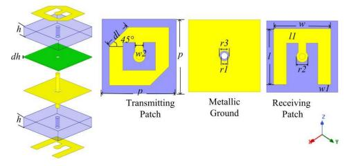
Figure 2. The schematic geometry of transmitarray unit cell.
