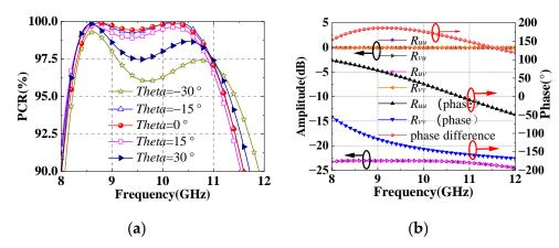
**Figure 7.** (a) The PCR of reflectarray with incident angle less than  $30^{\circ}$ . (b) The reflection amplitudes and phases in *u*-*v* coordinate.
