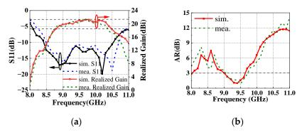
Figure 13. Simulated and measured results of GCPFTA (a) S11, realized gain and (b) AR.
