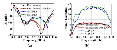
Figure 18. (a) The measured S11 of antennas. (b) The measured realized gain of antennas.
