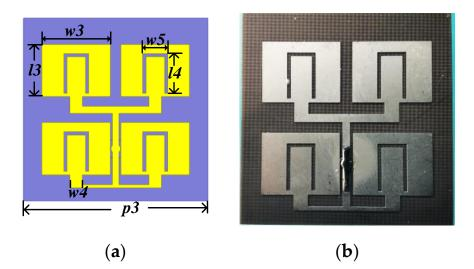
Figure 8. (a) The schematic geometry of planar feed antenna. (b) The fabricated planar feed antenna.
