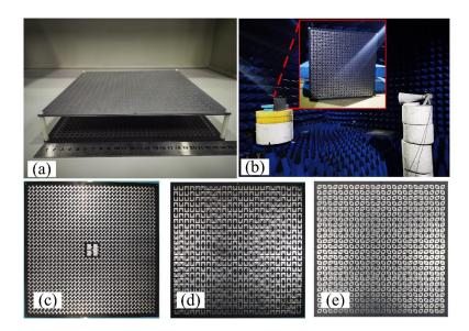
Figure 15. (a) The fabricated NCPFTA. (b) The measurement of NCPFTA in microwaves anechoic chamber. (c) The integrated reflectarray and planar feed with total size of 238 mm  $\times$  238 mm  $\times$  2.5 mm. (d) The bottom layer of transmitarray with size of 240 mm  $\times$  240 mm. (e) The top layer of transmitarray ray with size of 240 mm  $\times$  240 mm.
