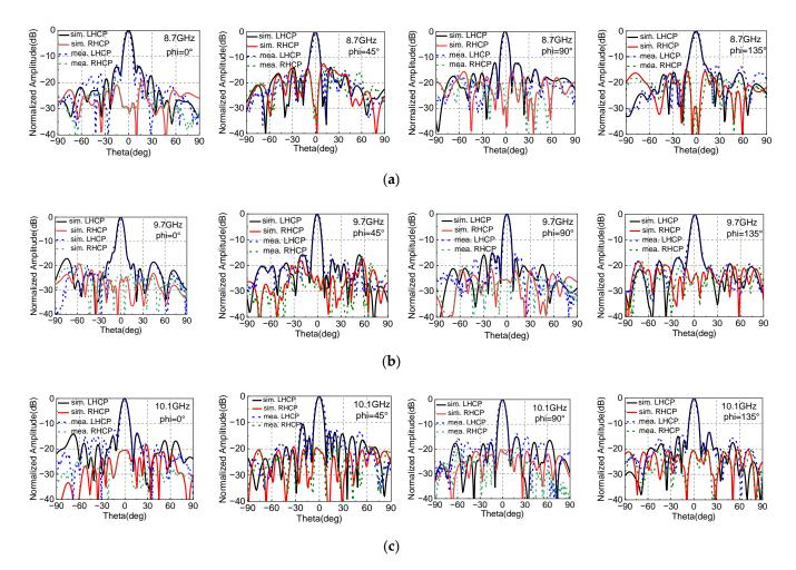
**Figure 17.** Simulated and measured radiation patterns in the phi =  $0^{\circ}$ , phi =  $45^{\circ}$ , phi =  $90^{\circ}$  and phi =  $135^{\circ}$  at (a) 8.7 GHz, (b) 9.7 GHz and (c) 10.1 GHz.
