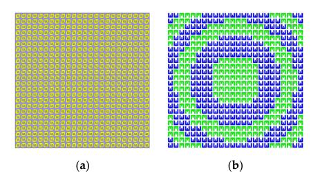
**Figure 11.** (a) The arrangement of  $24 \times 24$  anisotropic patches on the top layer of transmitarray with size of 240 mm × 240 mm. (b) The arrangement of  $24 \times 24$  E-shaped patches on the bottom layer of transmitarray with size of 240 mm × 240 mm.
