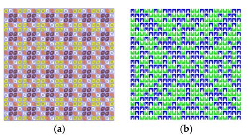
**Figure 14.** (a) The arrangement of  $24 \times 24$  anisotropic patches with size of  $240 \text{ mm} \times 240 \text{ mm}$ . (b) The arrangement of  $24 \times 24$  E-shaped patches with size of  $240 \text{ mm} \times 240 \text{ mm}$ .
