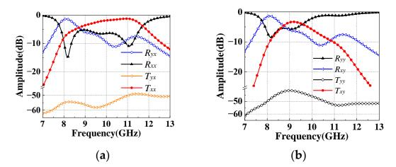
**Figure 20.** The amplitudes of co-polarized reflection, cross-polarized reflection, co-polarized transmission and cross-polarized transmission under (**a**) *x*-polarized and (**b**) *y*-polarized detection waves.
