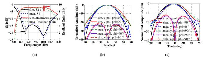
**Figure 9.** The simulated and measured (**a**) S11, realized gain, and radiation patterns at (**b**) 8.7 GHz and (**c**) 10 GHz.
