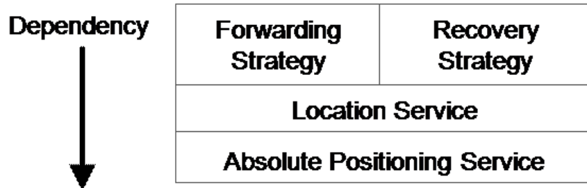
Figure 4: The components of a geographic routing algorithm
