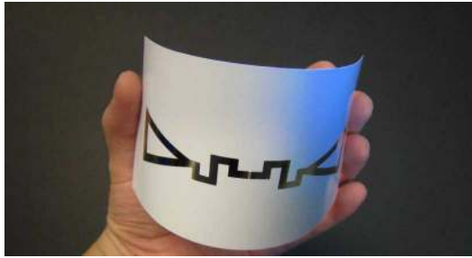
Fig. 9. Photograph of the conformal tag with a SWCNT film in the center.
