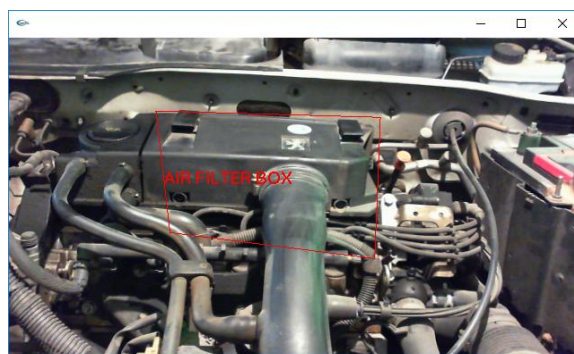
Fig. 16. Change air filter - step 1
