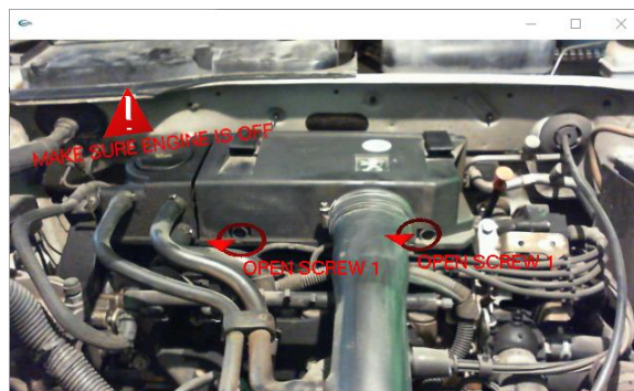
Fig. 17. Change air filter - step 2
