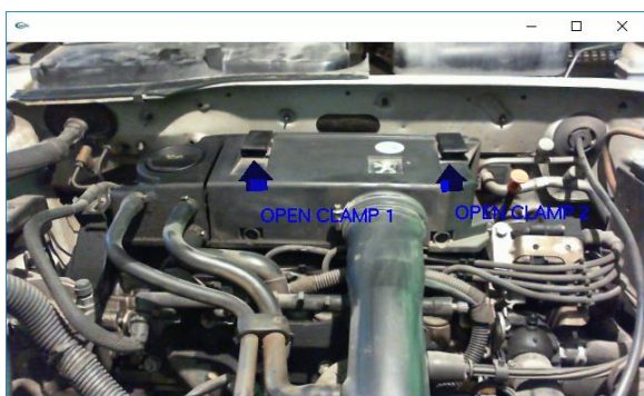
Fig. 19. Change air filter - step 3
