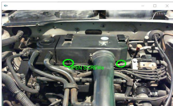
Fig. 18. Change air filter - step 2
