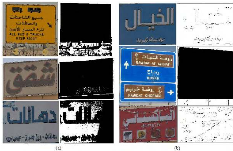
FIGURE 23. Examples of some bad images. (a) Misclassified text region in binary images. (b) Text detection is ambiguous in some image masks.
