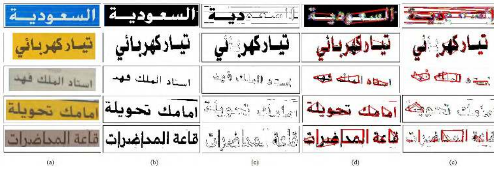
FIGURE 19. (a) Original images. (b) Binary images (c) Image masks (d) Extremal region detected in binary image (e) Extremal region detected in image mask.
