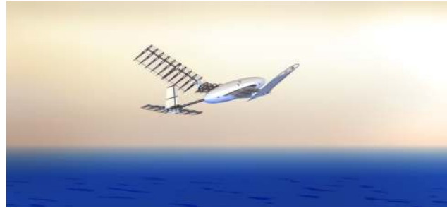
Fig. 1. Dual Aerial/Aquatic Flapping Vehicle Concept - Concept vehicle using in-line motion, an additional degree of freedom on a flapping wing, to provide the force necessary for propulsion in two fluids.
