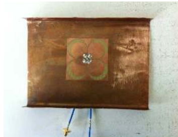
Figure 2. Photo of the fabricated antenna element.
