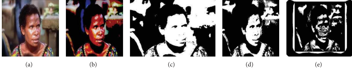
FIGURE 6: (a) Original image, (b) image of bit plane 8, (c) binarization of original image using mean threshold, (d) binarization of bit plane 8 with mean threshold, and (e) binarization of bit plane 8 with Niblack's method of local threshold.
