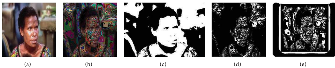
FIGURE 3: (a) Original image, (b) image of bit plane 5, (c) binarization of original image using mean threshold, (d) binarization of bit plane 5 with mean threshold, and (e) binarization of bit plane 5 with Niblack's method of local threshold.
