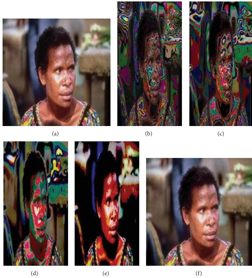
FIGURE 2: (a) Original image, (b) image of bit plane 5, (c) image of bit plane 6, (d) image of bit plane 7, (e) image of bit plane 8, and (f) amalgamated image of bit planes 5, 6, 7, and 8.
