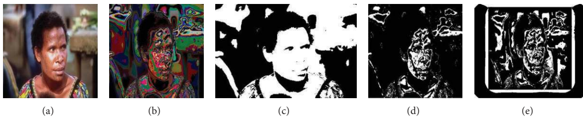
FIGURE 4: (a) Original image, (b) image of bit plane 6, (c) binarization of original image using mean threshold, (d) binarization of bit plane 6 with mean threshold, and (e) binarization of bit plane 6 with Niblack's method of local threshold.
