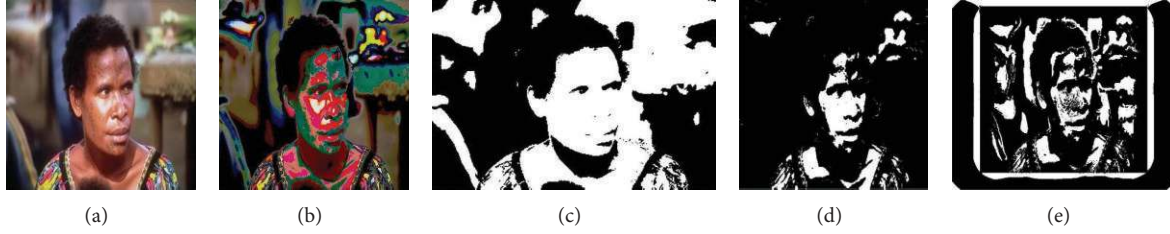
FIGURE 5: (a) Original image, (b) image of bit plane 7, (c) binarization of original image using mean threshold, (d) binarization of bit plane 7 with mean threshold, and (e) binarization of bit plane 7 with Niblack's method of local threshold.
