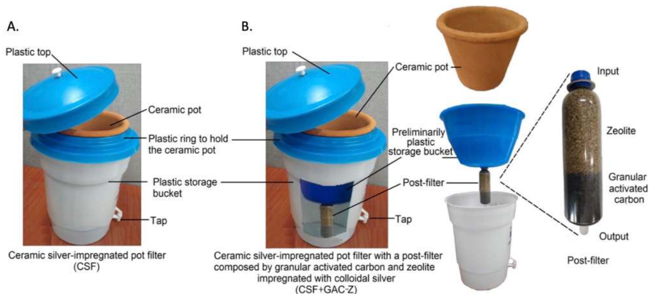
Figure 1. Ceramic-based point-of-use water treatment systems. (A) Ceramic silver-impregnated pot filter (CSF). (B) Ceramic silver-impregnated pot filter with a post-filter composed of granular activated carbon (GAC) impregnated with colloidal silver and zeolite (Z) (CSF + GAC-Z).
