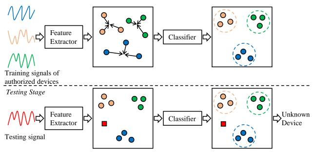
Figure 2. The open-set authentication of IoT devices.
