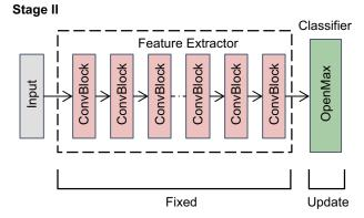
**Figure 3.** The training stages of the proposed framework. First, the feature extractor is trained by AAMSoftmax. Then, the OpenMAX classifier is updated with the fixed feature extractor.
