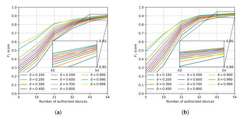
**Figure 11.** The  $F_1$  scores of softmax + OvA and AAMSoftmax + OvA with different  $\delta$  values. (a) Softmax+OvA; (b) AAMSoftmax+OvA.
