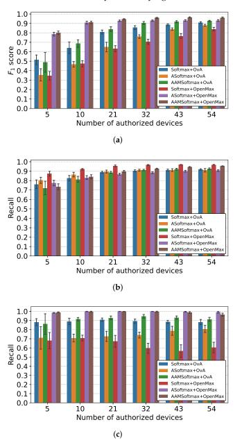
**Figure 10.** The performances of different combinations. (a)  $F_1$  score of all devices; (b) Recall of authorized devices; (c) Recall of unknown devices.
