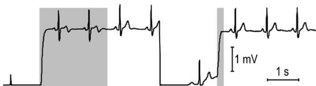
Fig. 6. ECG records obtained with the amplifier in Fig. 5 when operating the “fast-recovery” switches. Gray segments correspond to switches SW_{FR} , SW'_{FR} closed (see Fig. 5). In the first segment, the switches were manually operated to simulate an equipment startup. In the second segment, the switches were shortly closed, corresponding to a lead commutation. ECG amplitude is input referenced.
