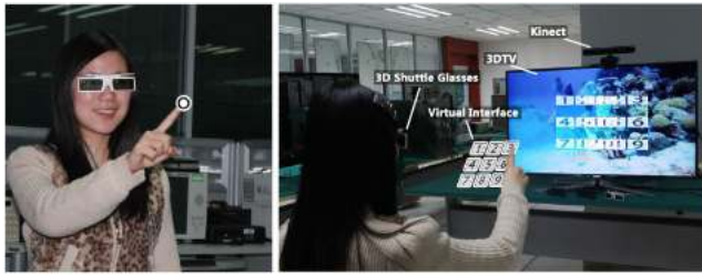
FIGURE 1. The proposed human-3DTV interaction system enables users sitting in front of the 3DTV to remotely control the television by directly touching the virtual interface with simple free-hand gestures.
