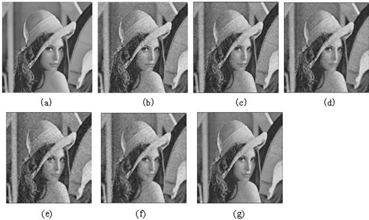
Figure 4 Image lena and experimental results. (a) Original image lena. (b) Gaussian white noising image. (c) Hyperbolic shrinkage in [15]. (d) MATS method in [14]. (e) Improved soft-threshold in [16]. (f) AdpMpMHard in [18]. (g) This article.
