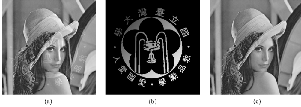
Fig. 5. Proposed algorithm recovers the linear-gradient watermarked image. (a) Watermarked image with PSNR = 30.97 dB. (b) Linear-gradient watermark with r = 12 and \theta = 220^\circ . (c) Recovered image with PSNR = 47.22 dB in 783.30 s ( r_{\text{final}} = 8 and \theta_{\text{final}} = 233^\circ ).
