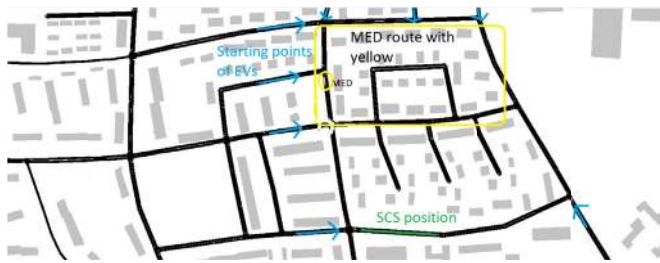
Fig. 5. Section of the Erlangen city map used to conduct the simulations. The MED route is marked in yellow. The position of the SCS is marked in green. The arrows in cyan point at the journey starting points of the EVs. The buildings are represented for the Non-Line of Sight (NLOS) links to be considered in the V2V communication.
