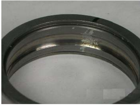
FIGURE 22: Picture of outer race fault bearing.
