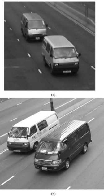
Fig. 1. Vehicle occlusion. (a) Same lane and (b) adjacent lanes.
