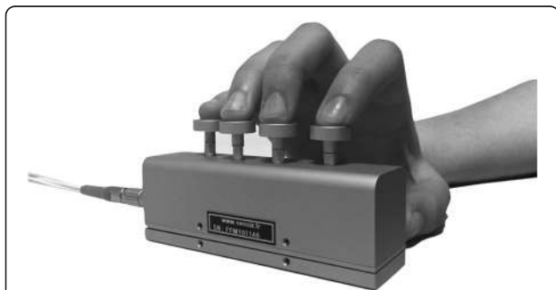
Fig. 1 The Finger Force Manipulandum (FFM). Index, middle, ring and little finger each apply forces on a spring-loaded piston. Two types of tasks were implemented: continuous force tracking and finger tapping. Forces applied by each finger were recorded via a CED interface (not shown) and used for real-time visual feedback and for performance analysis
