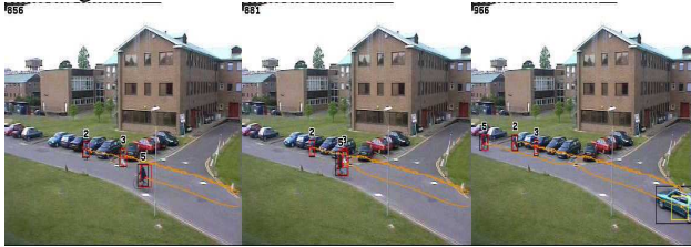
Figure 9: Example of dynamic occlusion reasoning for PETS2001 dataset 2 camera 2.
