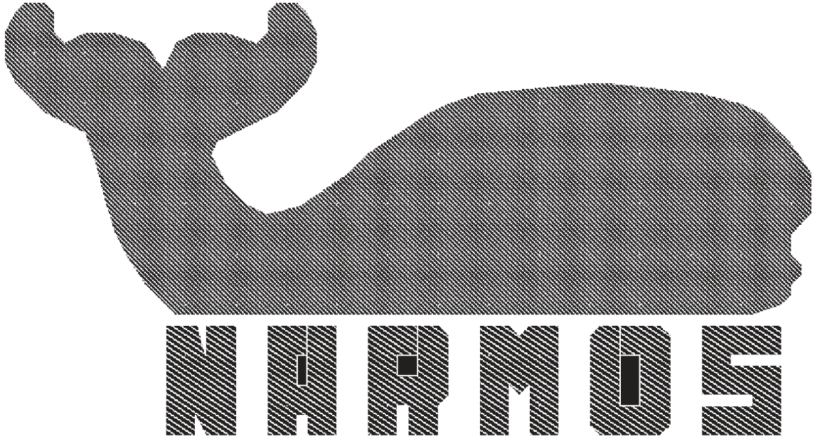
Figure 7: Sample IC logo implemented in AMI C5N that passed DRC check
