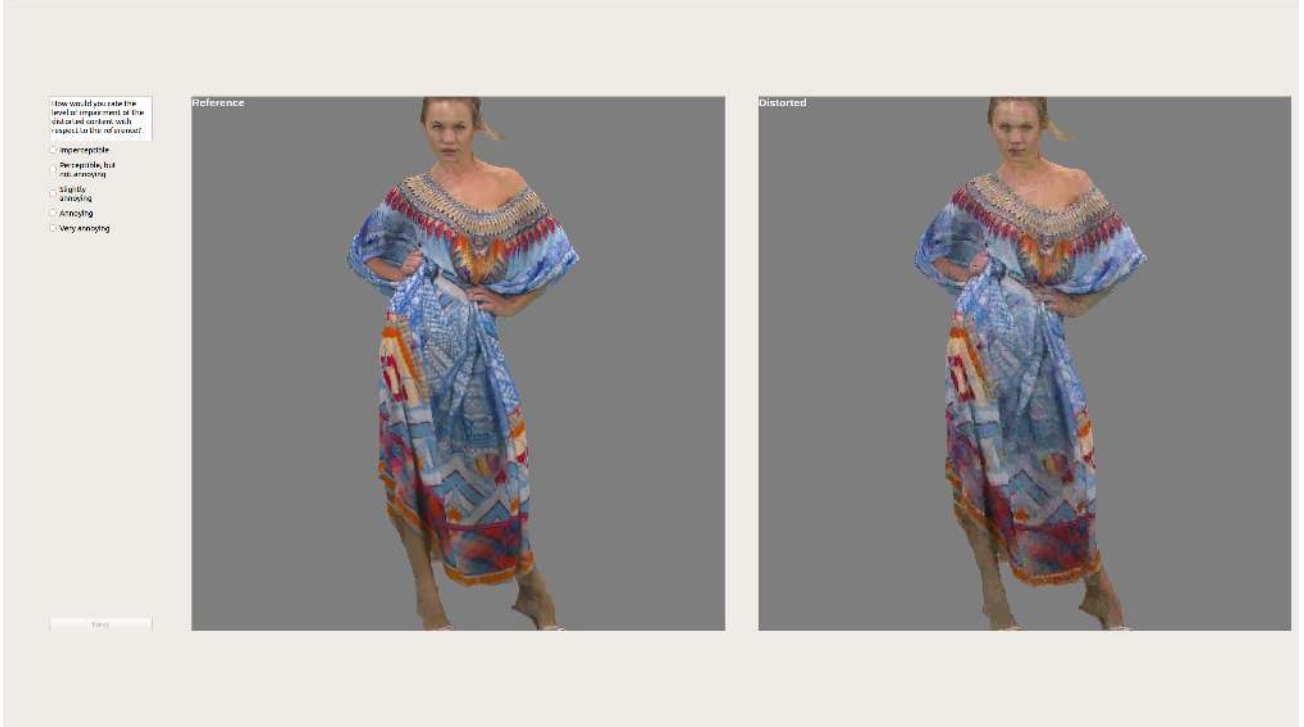
Figure 4. A screenshot of the GUI presenting the reference longdress content at the left, and its compressed version using octree-depth equal to 10 and JPEG quality parameter equal to 10.
