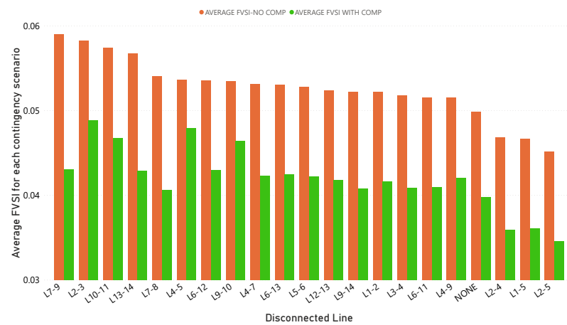
Figure 6. Fourteen-bus-bar system: FVSI for contingencies with no compensation vs. contingencies with optimal compensation.
