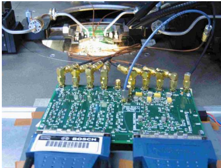
Figure 4.12.: Measurement setup for the I-Q transceiver module.
