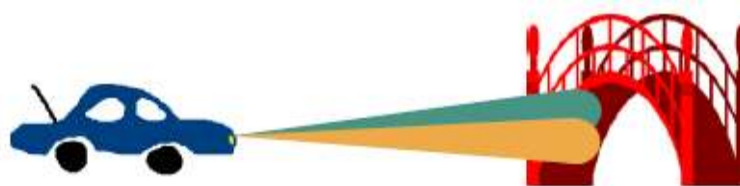
Figure 1.10.: Beam steering in elevation to detect a bridge.
