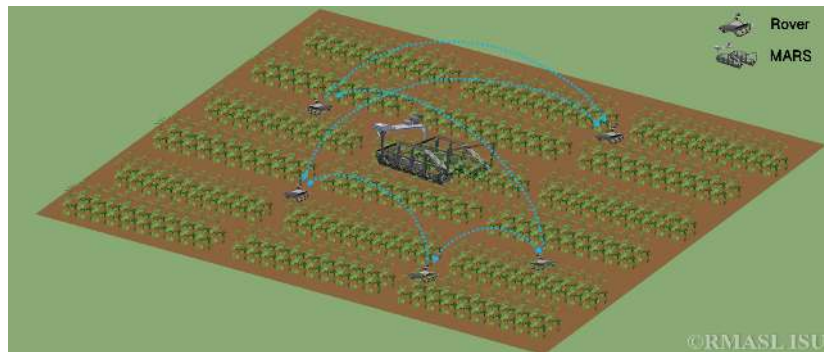
Figure 1. Deployment strategy of robotic phenotyping system.
