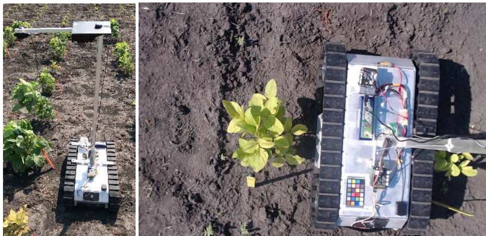
Figure 6. Image of the soybean canopy from the overhead camera mounted on the rover.
