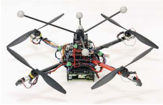
Fig. 1: Picture of the holocopter prototype. The four propeller groups are slightly tilted. The red bar indicates the positive direction of the \mathbf{X}_B holocopter body axis
