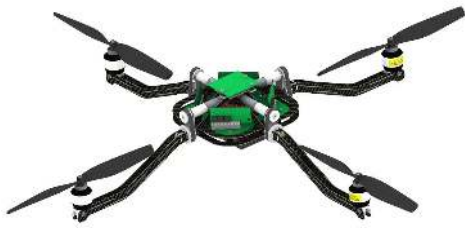
Fig. 26: CAD image of the new prototype with improved mechanics, actuation system, electronics and an overall reduced mass and inertia
