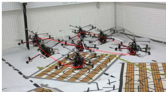
Fig. 24: Third experiment. Overlay of several snapshots of the holocopter while performing eight-shape trajectory
